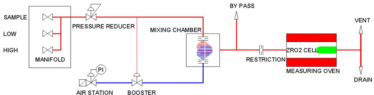
**Fig.1 Schematic typical residual oxygen content analyzer**
