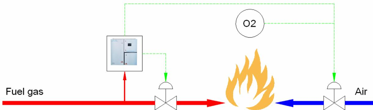
In case large fluctuations in the fuel gas are expected. The wobble index of the gas flow can be stabilized using the fast responding Wobbe Index signal.
