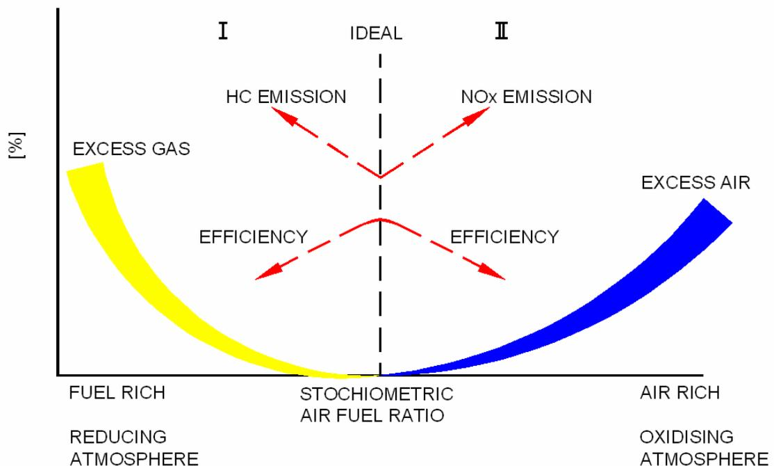
The table above shows the efficiency vs the amount of air / gas introduced to the combustion process. The black dotted line indicates the stoichiometric air fuel ratio (the exact amount of air required for the combustion of 1m<sup>3</sup> of gas under normal conditions), and is the most efficient way to combust your product and have lowest possible NO<sub>x</sub> or HC emission.
